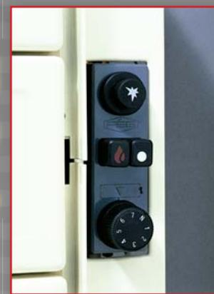
The CRH 6 Self Energized Gas Control Valve is a multi-functional control incorporating an ON-OFF valve, a thermoelectric flame supervision device, and a mechanical thermostat for room temperature regulation as well as optional – a pressure governor and a piezo igniter with ignition interlock. Max. and min. gas rate are adjustable.
